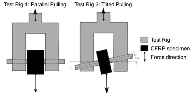
Fig. 3: Test setups 1 and 2 for residual strength test of the bore channel after a drilling operation.
