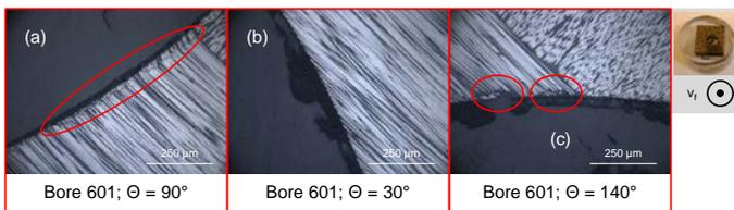
Fig. 2: Subsurface damages for different fibre orientations  $\Theta$  [6].
