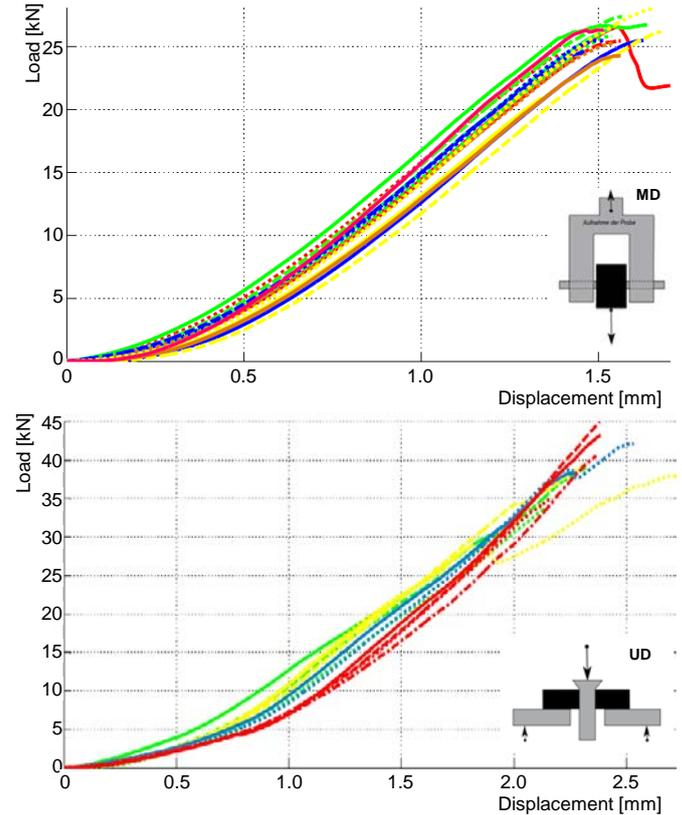
Fig. 7: Exemplary load-displacement graphs for test setup 1 with woven and test setup 3 with unidirectional CFRP.
