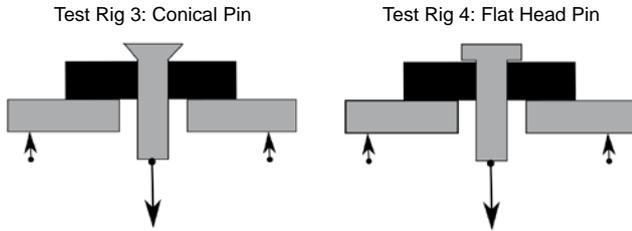
Fig. 5: Test setups 3 and 4 for residual strength test of the bore exit after a drilling operation.
