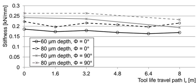
Fig. 12: Exemplary stiffness for Elliptical Cone Test (Test 6) and Drill Model 8 loaded in reverse feed direction.
