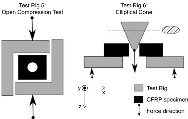
Fig. 6: Test setups 5 and 6 for mechanical strength of drilled CFRP specimens.
