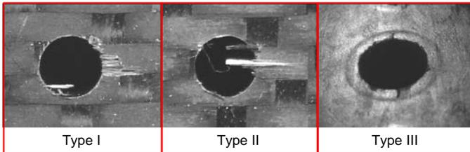
Fig. 1: Types of delamination.
