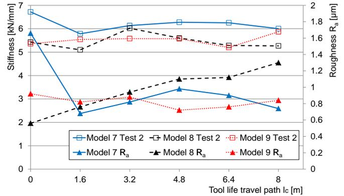
Fig. 10: Mechanical strength for Tilted Pulling Test (Test 2) and roughness of bore wall.
