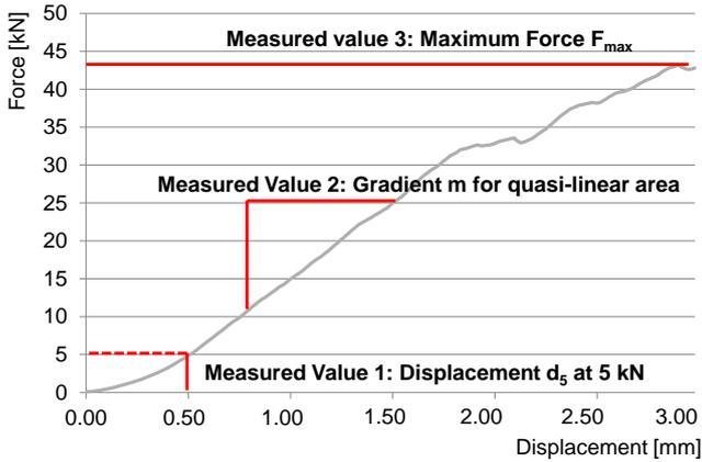
Fig. 8: Analyse scheme for load-displacement curve.
