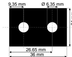
Fig. 4: Design of CFRP specimen for test setups 1 and 2.
