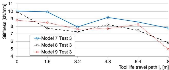
Fig. 11: Exemplary stiffness for Conical Pin Test (Test 3) loaded in reverse feed direction.
