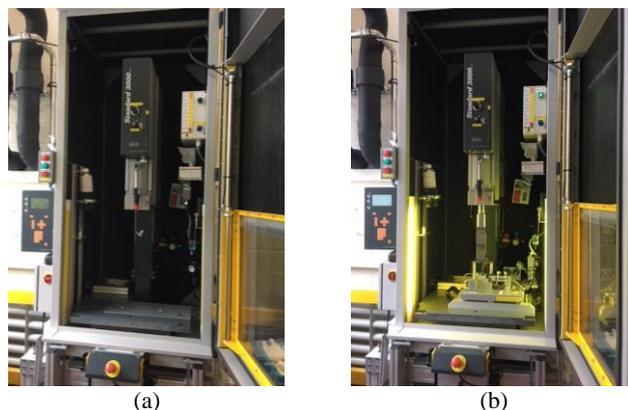
Fig. 1. Ultrasonic welding machine (a) idle (empty), (b) with installed tools (Geberit Produktions AG, Jona, CH).
