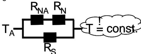
FIGURE 2. Simplified thermal equivalent circuit diagram of the ball screw system,  $R_S$ : thermal resistance spindle side,  $R_N$ : thermal resistance of the nut,  $R_{NA}$ : convective thermal resistance of the nut to the ambient air.
