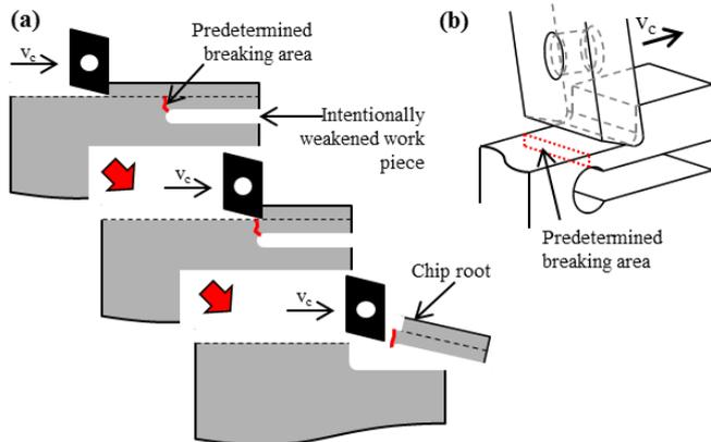
Fig. 5. Sequence of chip root generation: (a) Side view; (b) 3D.
