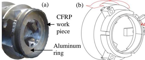
Fig. 2. (a) Test rig for orthogonal cutting tests; (b) schematic illustration.
