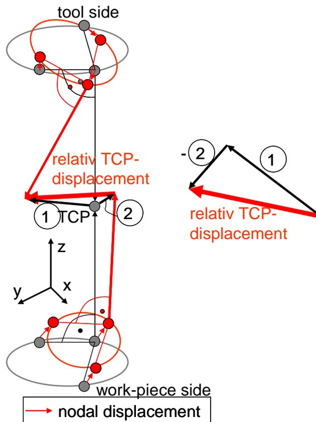
Figure 2: calculating relative TCP-displacement
