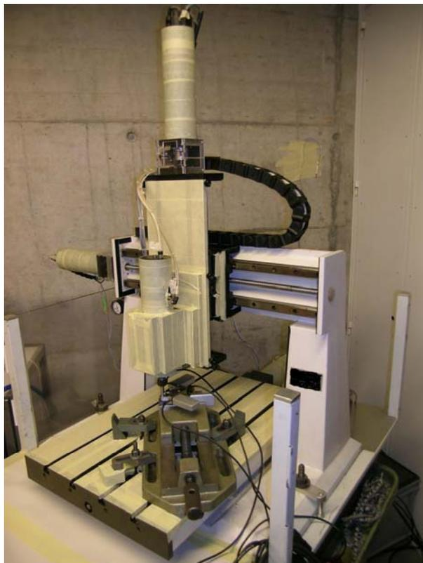
Figure 5: Three-axis milling machine
