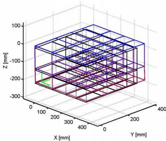
Figure 6: Calculated TCP-displacements in workspace, before compensation distortion is shown with an augmentation factor of 6'000
