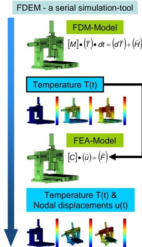
Figure 1: schematic of the FDEM; here:  $M$  = FDM model matrix,  $d\bar{T}$  = temp. change,  $\bar{H}$  = constant vector,  $C$  = FEA model matrix,  $\bar{F}$  = thermal forces
