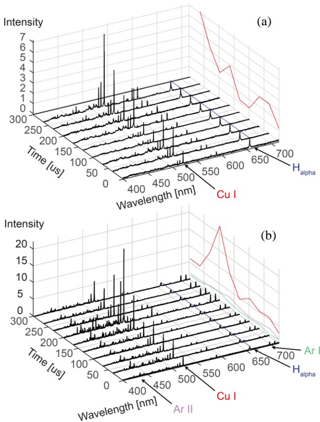
Figure 11: (a) Spectrum of single discharge in air; (b) Spectrum of single discharge in argon
