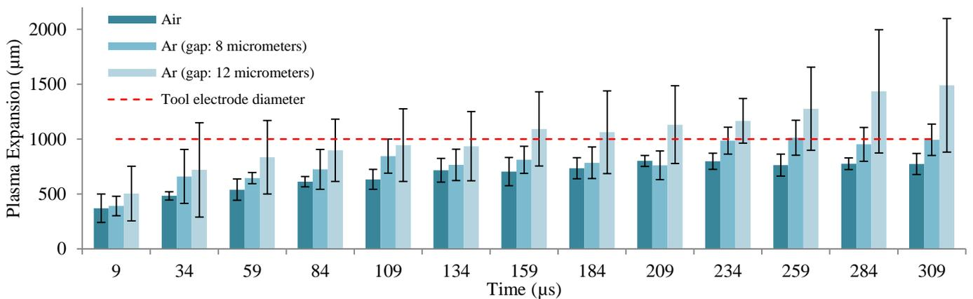
Figure 10: Plasma expansion in function of time for discharges in air and argon
