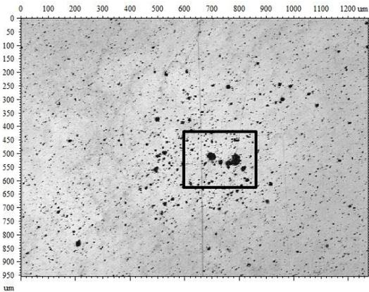
Figure 7: Craters left by a 316  $\mu\text{s}$  single discharge in argon (U = 250 V; I = 20 A; Positive tool electrode)
