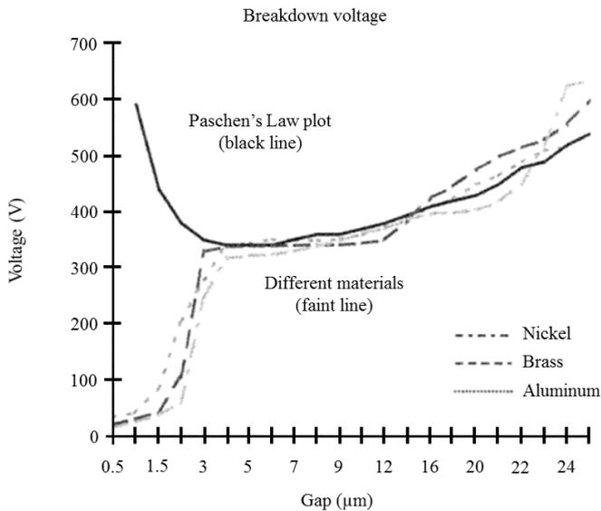
Figure 1: Breakdown voltages in air versus gap at atmospheric pressure for different electrode materials [4]
