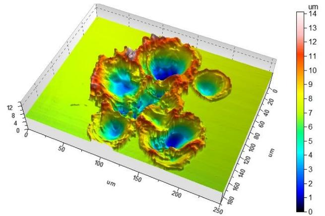
Figure 4: Several craters made in air by spark with 75  $\mu\text{s}$  duration (U = 250 V; I = 20 A; Negative tool electrode)
