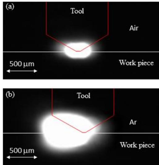
Figure 9: (a) Plasma expansion in air; (b) Plasma expansion in argon
