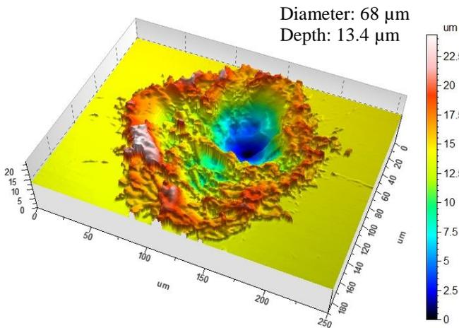
Figure 3: Single crater made in air by spark with 75  $\mu\text{s}$  duration (U = 250 V; I = 20 A; Negative tool electrode)
