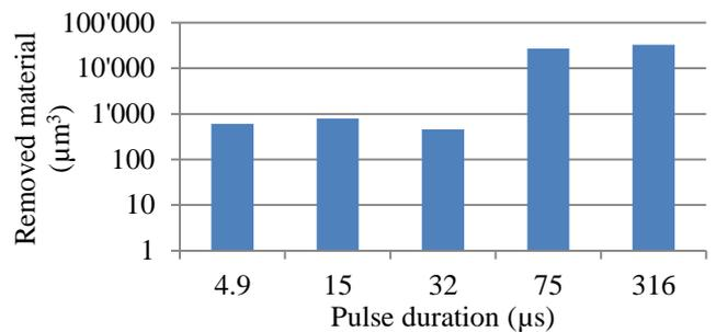
Figure 6: Evolution of the averaged material removal in function of time (U = 250V; I = 20 A; Negative tool electrode)
