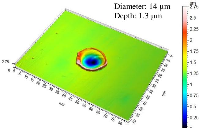
Figure 2: Single crater made in air by spark with 4.9  $\mu\text{s}$  duration (U = 250 V; I = 20 A; Negative tool electrode)
