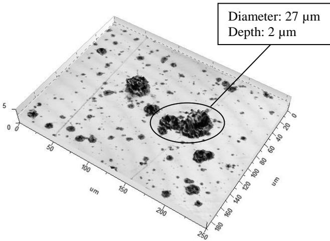
Figure 8: Amplification of craters from Figure 7 left by a 316  $\mu\text{s}$  single discharge in argon (U = 250 V; I = 20 A; Positive tool electrode)
