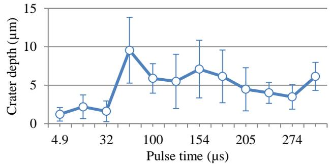
Figure 5: Evolution of the crater depth average during the time in air (U = 250 V; I = 20 A; Negative tool electrode)
