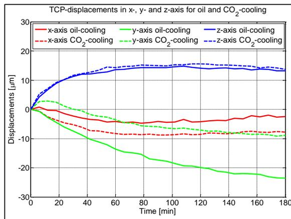
Fig. 4. measurement of the thermal displacements in x-, y- and z-direction over time as a function of the cooling medium oil or  $\text{CO}_2$
