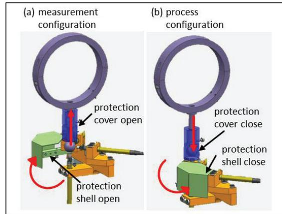
Fig. 3. (a) measurement setup with protection cover and shell opened in the measurement configuration; (b) measurement setup with protection cover and shell closed during the use of oil and CO<sub>2</sub>.
