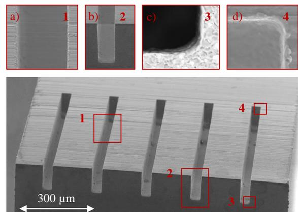
**Figure 7** Workpiece eroded using 2 Cu electrodes.
