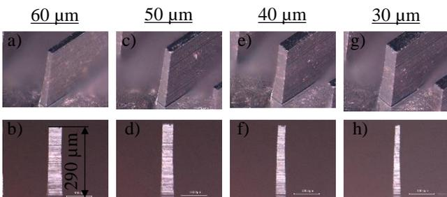
**Figure 5** Burr-free bars in WCu with high aspect ratio  $AR$ ; a) & b) flawless bars having an  $AR = 5$ ; c) – f) deviation from width of  $\sim 7\ \mu\text{m}$ ; g) & h) conical shape pronounced.
