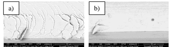
**Figure 3** Impact of milling direction when machining WCu; a) surface defects in up-milling; b) enhance of surface quality in down-milling.
