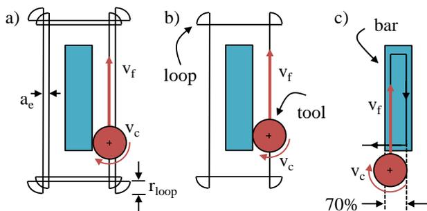
**Figure 2** Milling Strategy for burr-free machining; a) roughing to achieve final dimension; b) deburring of lateral burrs; c) deburring of top burrs.
