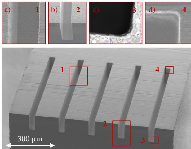
Figure 8 Workpiece eroded using 5 WCu electrodes.
