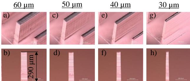
**Figure 4** Burr-free bars in Cu with high aspect ratio  $AR$ ; a) & b) flawless bars having an  $AR = 5$ ; c) – f) deviation from width of  $\sim 7\ \mu\text{m}$ ; g) & h) conical shape pronounced.
