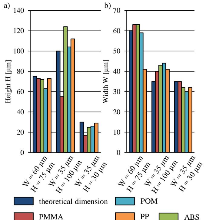
Figure 10 Influence of different plastic types to resultant dimensions of micro-bars when applying variotherm technology; a) achievable height H; b) achievable width W.
