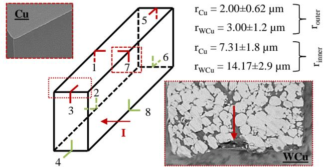
**Figure 6** Representation of edge measuring locations.
