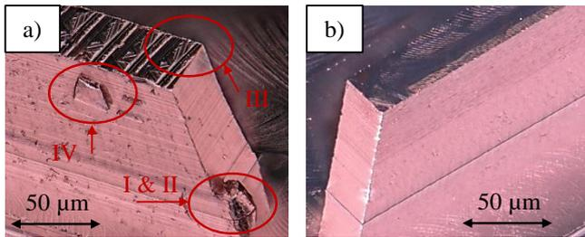
**Figure 1** Burr formation when micro-milling Cu; a) observation of four burr types; b) burr-free micro-structure.
