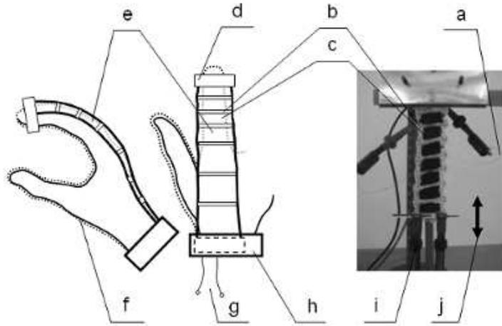
**Fig. 2.** L.: Schematic of a chain-like actuator for the index finger. R.: Demonstrator. *a*: connector, *b*: fixture, *c*: dielectric elastomer film sandwiched by compliant electrodes, *d*: ring, *e*: chain-like actuator, *f*: rubber glove, *g*: power supply, *h*: nylon band, *i*: mass, *j*: output direction.
