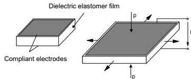
**Fig. 1.** Working principle of a dielectric elastomer actuator.
