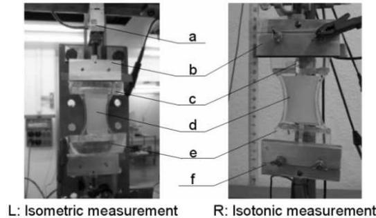
**Fig. 4.** Setup of the *isometric* (L.) and *isotonic* (R.) measurement. *a*: force transducer, *b*: aluminium clamps, *c*: connectors, *d*: dielectric elastomer applied with compliant electrodes, *e*: plastic film, *f*: mass.
