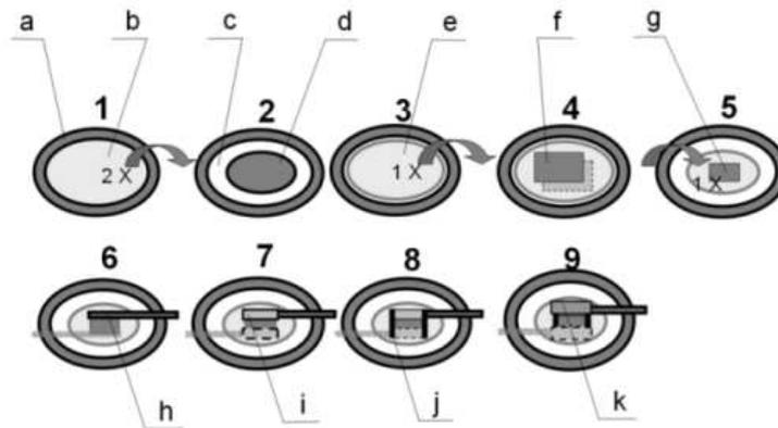
**Fig. 3.** Manufacturing process of a one-layer actuator element. *a:* torus, *b:* dielectric elastomer film, *c:* talc, *d:* circular mask, *e:* dielectric elastomer film, *f:* electrode, *g:* compliant electrode, *h:* connector, *i:* protective film, *j:* strips, *k:* plastic film.
