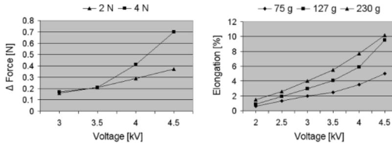
**Fig. 5.** L. *Isometric measurement*: The variation of contractile forces vs. the voltage under the initial forces of 2 and 4 N. R. *Isotonic measurement*: the elongation vs. the voltage under the masses of 75, 127 and 230 g.
