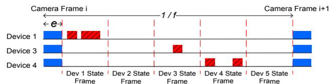
**Figure 2. State information transfer example with  $M$  set to 5 and with devices 1, 3, and 4 (rows) present. One interval between camera frames  $i$  and  $i+1$  is shown. Blue cells are IR flashes to be detected by the camera; red cells are IR flashes to be detected by the IR receiver.**
