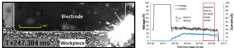
Figure 3: Time synchronised visual and electrical information of the EDM spark. To correlate the electrical information of the sparks with their photographs, time synchronisation is performed through oscilloscope auxiliary output, triggered based on current channel, where steady-state or any chosen part of the process is acquired.
