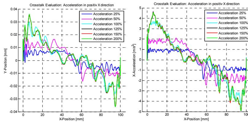
Figure 3: Crosstalk and acceleration on a set of positioning cross-grid measurements
