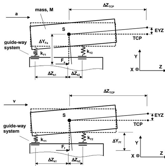
Figure 2: Schematic of the inertia (top) and friction (bottom) tilt effects on the TCP
