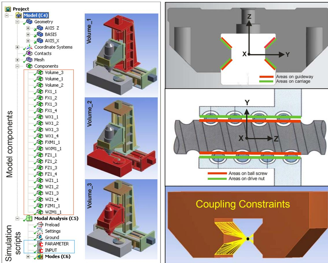
Figure 1: Illustration of the component definition in an ANSYS Workbench simulation model
