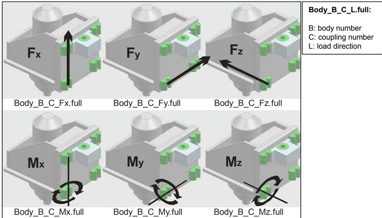
Figure 2: Load definition for the coupling locations: one .full file per load direction
