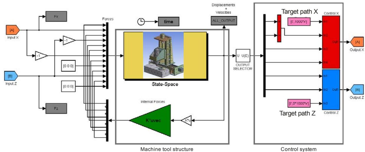
Figure 6: The complete Simulink model containing the model of the machine tool structure, as well as two basic cascaded control systems for the two motion directions X and Z.
