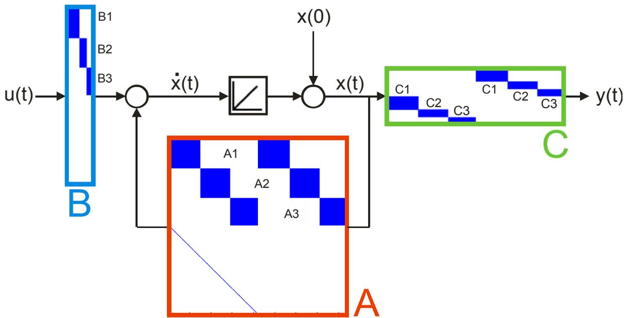
Figure 3: Combination of the three state-space systems  $(A_1, B_1, C_1, D_1)$ ,  $(A_2, B_2, C_2, D_2)$  and  $(A_3, B_3, C_3, D_3)$  into one global state-space system by assembling the individual matrices
