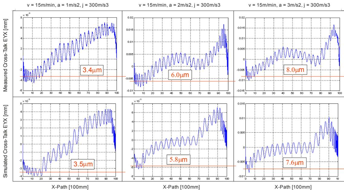
Figure 10: Measured and simulated cross-talk values by variable acceleration values
