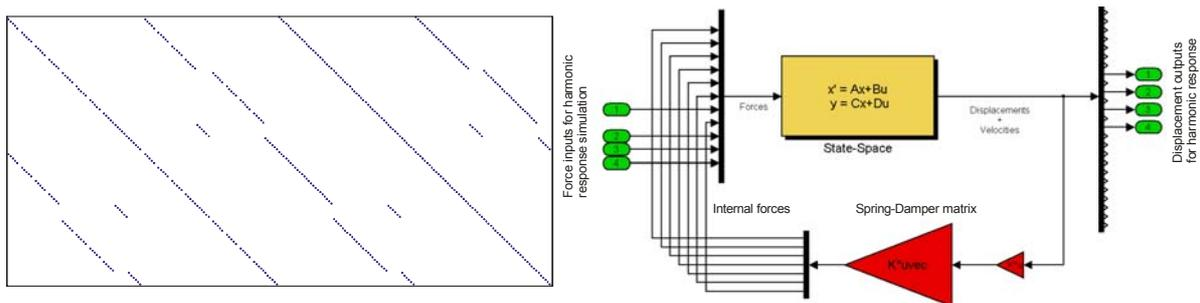
Figure 4: “Spring-Damper” matrix (left) and Simulink model (right) for a harmonic response simulation including the assembled state-space system and the additional Spring-Damper matrix specifying the internal coupling characteristics
