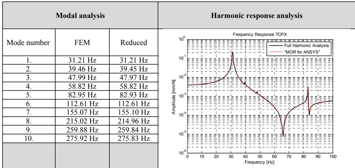
Figure 7: Comparison between full ANSYS simulation and reduced MATLAB simulation
