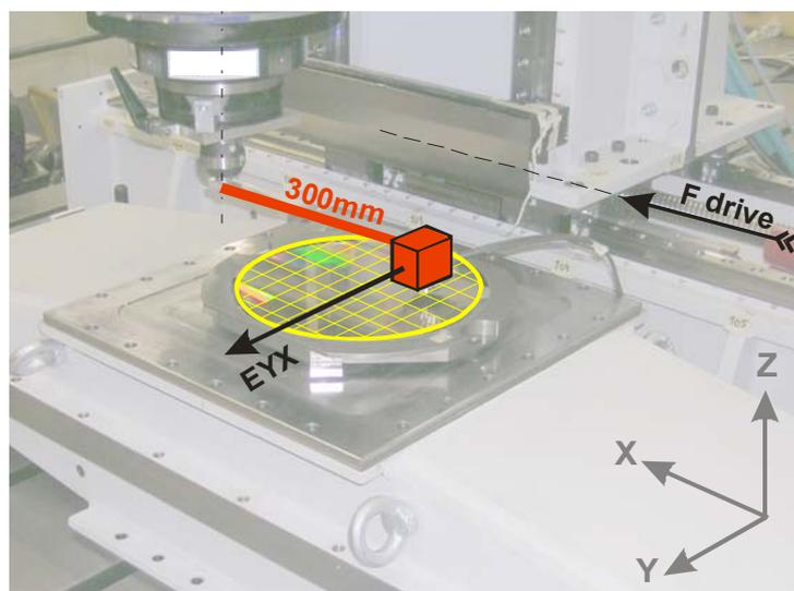
Figure 9: Cross-grid measurement set-up
