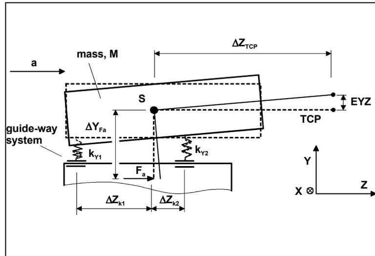
Figure 8: Schematic of the inertia tilt effects on the TCP
