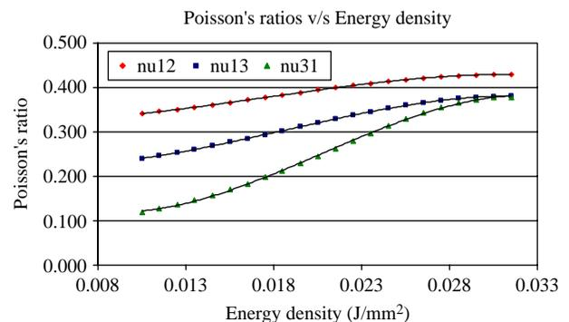
803 MPa and 0.408 for the Young's modulus, Shear's modulus and Poisson's ratio, respectively. These values are obtained for a maximum apparent density (mass density) equivalent to 977 kg/m<sup>3</sup>. Uniaxial tensile tests were also performed on the laser sintered dogbone coupons to compare the two characterization techniques, indicating that a good agreement exists between them, at least for the measurements of the Young's modulus along the dogbone axis (~2.4 GPa).
