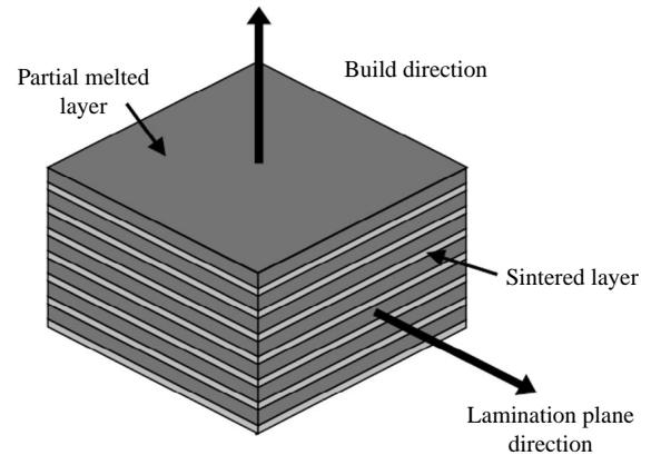
increases. In the present study, the material structure is associated to a hexagonal crystal, which is completely characterized by five independent elastic constants, representing a transversely isotropic behavior. According to the symmetry of this crystal, the notation adopted for the orthogonal main directions is shown in Figure 5.
