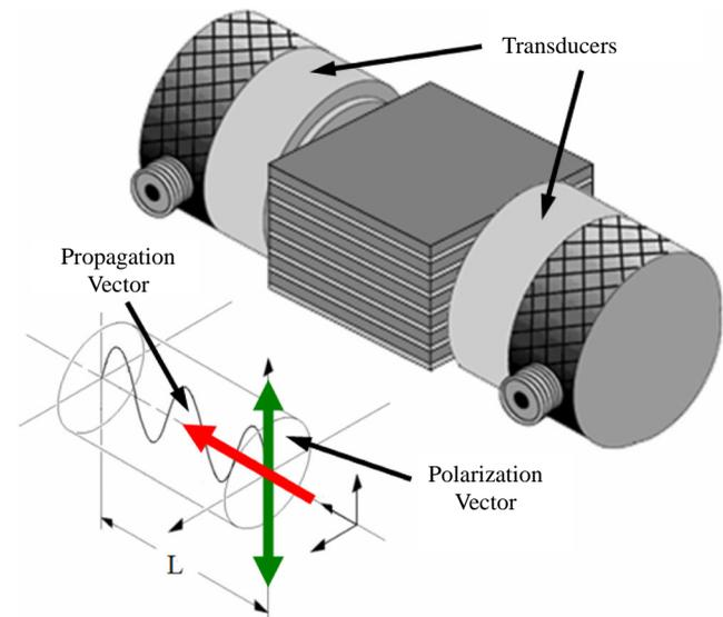
in Figure 9). In addition, the transducers delay time  $t_r$  was registered. Then, using the samples length  $l$  for a particular direction between parallel faces, the wave velocity can be calculated as follows:
