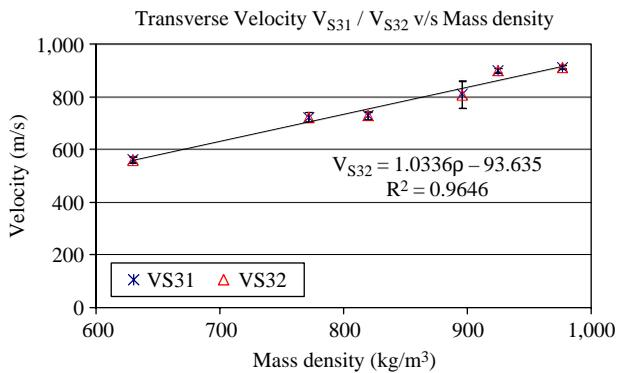
**Figure 15** Transverse velocities with polarization vector contained inside the lamination plane and perpendicular to the propagation vector
