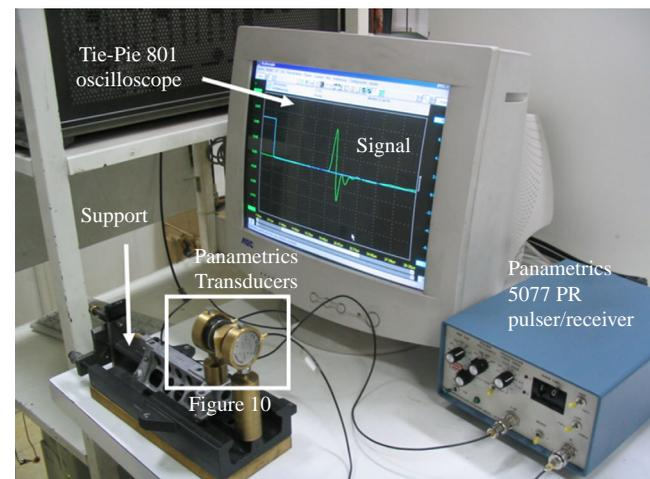
**Figure 10** Ultrasonic shear wave measurement setup
