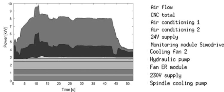
Figure 1 Power measurement of machining a drive shaft on a turning machine with process cooling by compressed air
