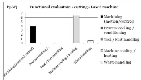
Figure 6 Functional evaluation of a laser machine
