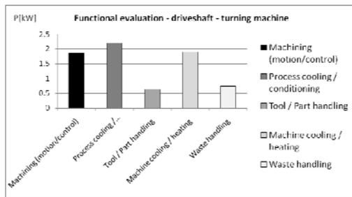
Figure 5 Functional evaluation of a drive shaft on a turning machine
