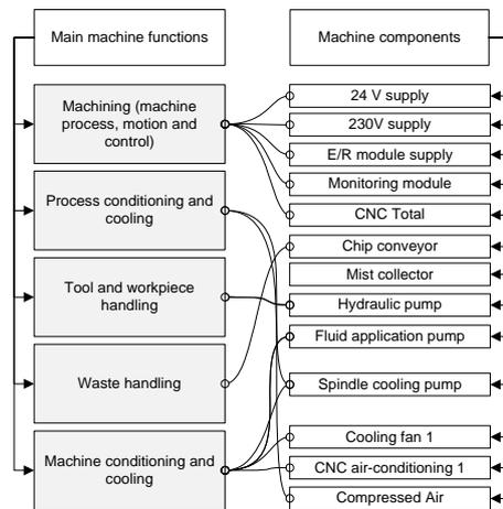
Figure 2 Main machine tool functions and its example components for a lathe
