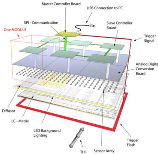
Figure 5. Principle setup of the MightyTrace
