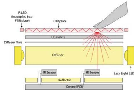
Figure 7. IR-sensors in the LC-screen
