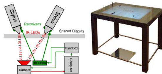
Figure 3. Principle setup of InfrActables and its realization
