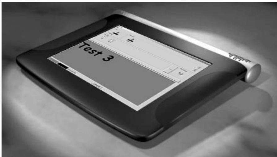
Figure 1. InnoPlan-Pad, the individual interaction unit of the InnoPlan-system
