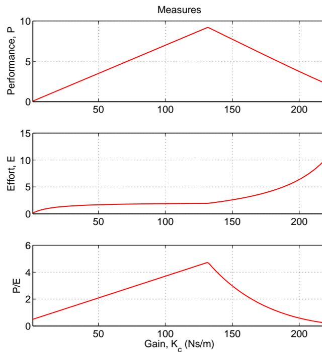
Figure 4: Measures obtained with the direct velocity feedback.
