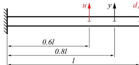
Figure 3: Cantilever beam model.
