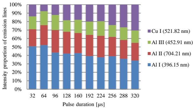
Figure 4: Ratios of intensity lines of electrical discharges with anode tool
