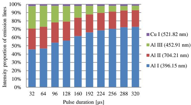
Figure 5: Ratios of intensity lines of electrical discharges with cathode tool
