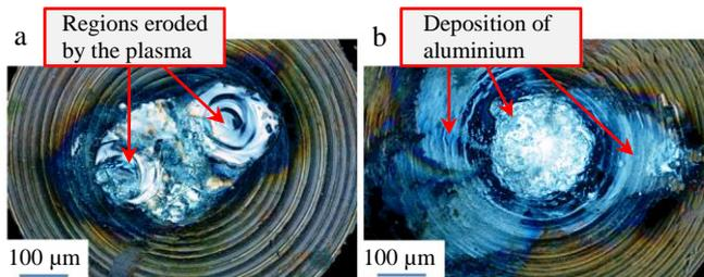
Figure 8: (a) Anode tool electrode; (b) Cathode tool electrode
