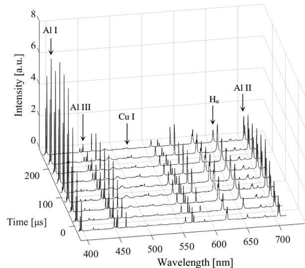
Figure 3: Emission spectra of a single electrical discharge with cathode tool
