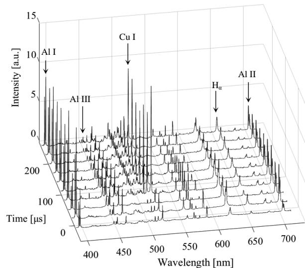
Figure 2: Emission spectra of a single electrical discharge with anode tool
