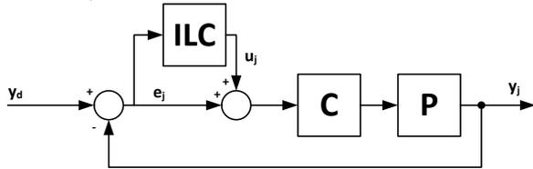
Fig. 1. General application scheme of the ILC algorithm.
