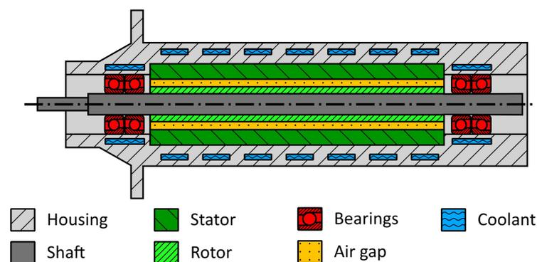
Figure 1: Generic representation of the modeled spindle with the implemented macro-models shown in different colours [4].
