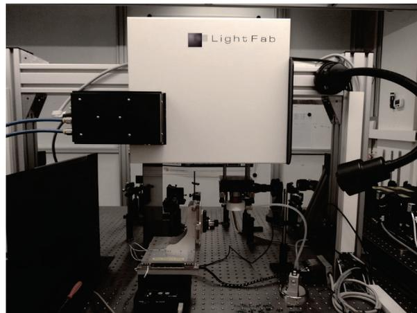
Figure 2. Experimental setup used to generate micro cutting tool geometries.
