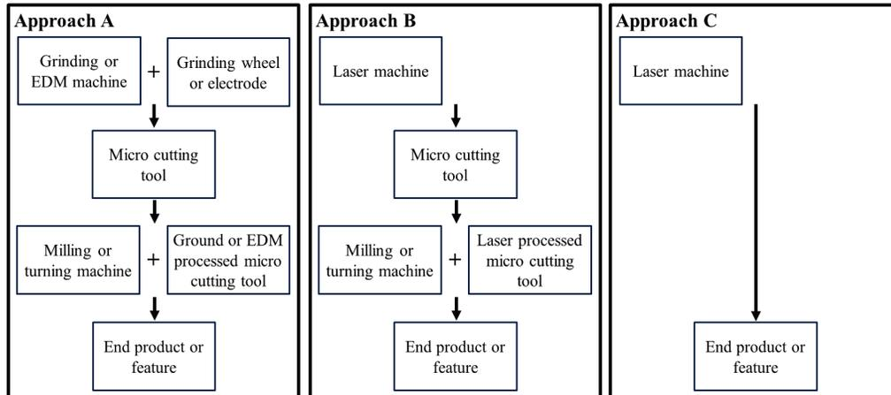
Figure 1. Different approaches and sequences needed to manufacture a product or feature.
