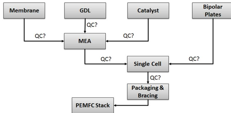
Figure 1: General Production Scheme of a PEMFC Stack
