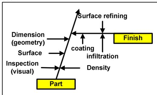
Figure 6: Q-elements of part and finishing
