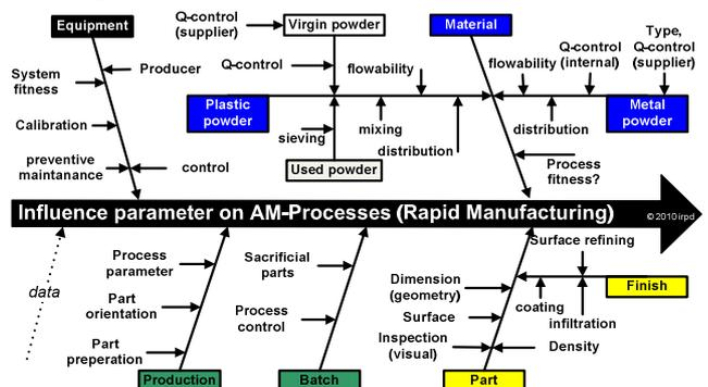
Figure 1: Parameter of production chain AM processes
