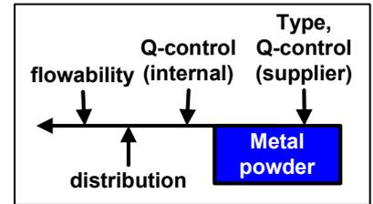
plastic powder, because metal powders are usually used in SLM processing as delivered and no significant aging is recognized. However, the part producer ('service bureau') is responsible for the quality of the used powder and the following data should be documented for quality reasons: production identification (e.g. Charge), Powder particle size distribution (d10/d50/d90), flowability (if accessible), applied sieving;
