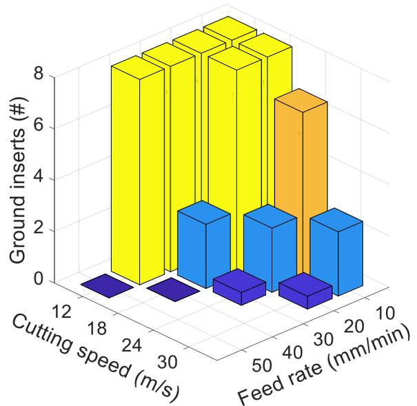
Fig. 10: Maximum dressing interval until temperature exceeds maximum.
