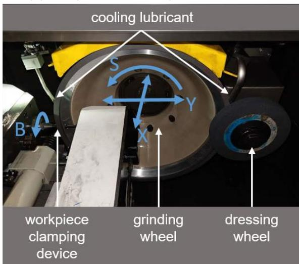
Fig. 3: Overview of cup wheel grinding machine.
