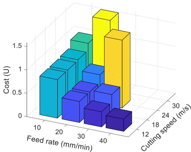
Fig. 11: Calculated costs using equation (2) as a function of feed rate and cutting speed.
