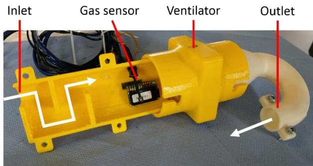
Fig. 6: Experimental setup of a gas sensor.
