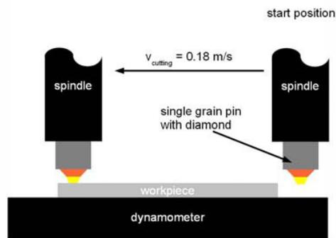
Fig. 2. Experimental Setup
