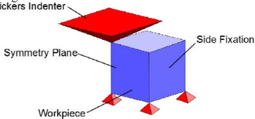
Fig. 4. Vickers Hardness Simulation
