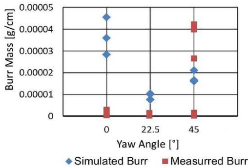
Fig. 6. Simulated and experimental burr generation rate
