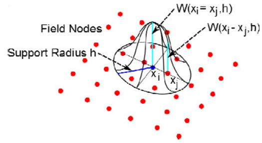
Fig. 1. SPH discretization
