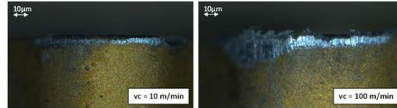
Fig. 8. Tool flank wear after cutting Titanium with (a)  $v_c = 10$  m/min; (b)  $v_c = 100$  m/min and 0.2 m cutting length.
