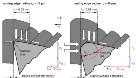
Fig. 2. Tool load on the cutting edge with elastic surface deflection with cutting edge radius  $r_n$  (a) 10 $\mu$ m; (b) 40 $\mu$ m [8].
