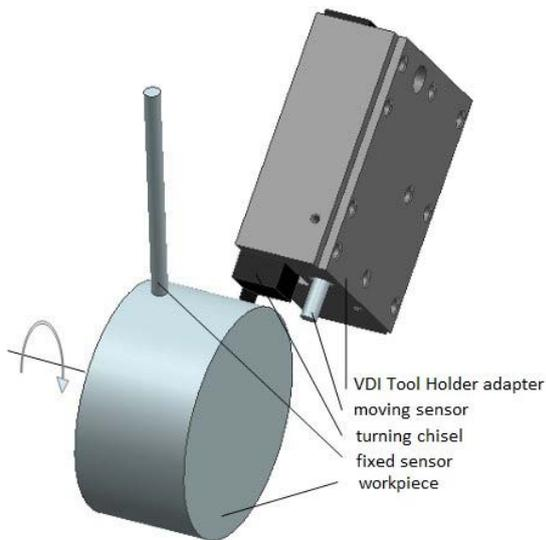
Fig. 4. Model of measuring set-up.
