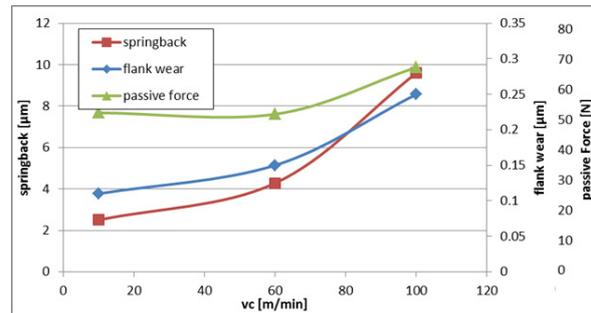
Fig. 9. Influence of the springback on the flank wear and the passive forces when cutting Ti6Al4V.
