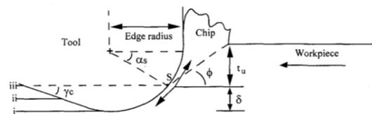
Fig. 1. Cutting with material separation point on edge with 3 recover scenarios [2].
