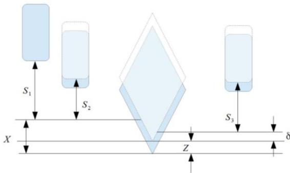
Fig. 3. Principle measuring set-up including Sensors 1-3 and cutting insert
