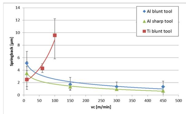
Fig. 6. Overview of the springback with sharp and blunt tool in Aluminium and Titanium machining.
