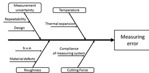
Fig. 5. Ishikawa diagram of the measuring error in springback measurements.
