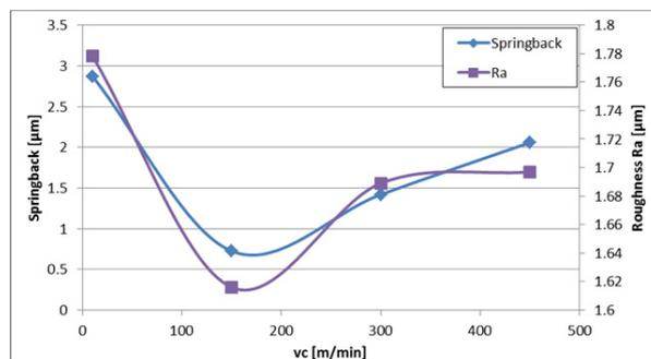
Fig. 7. Influence of the springback on the surface roughness  $R_a$  when cutting with wiper geometry AlMg1SiSn,  $f = 0.3$  mm/rev,  $a_p = 0.05$  mm
