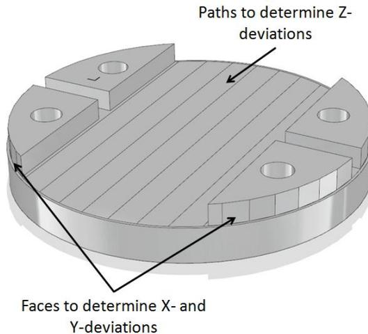
**Figure 1:** Proposed thermal test piece.
