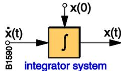
Figure 15. Integrator block as the representative of the solution procedure for an ordinary differential equation
