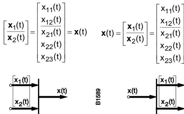
Figure 8. Merging and demerging of signals and signal vectors
