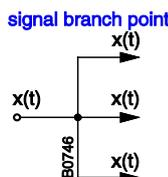
Figure 9. Branching of signals and signal vectors
