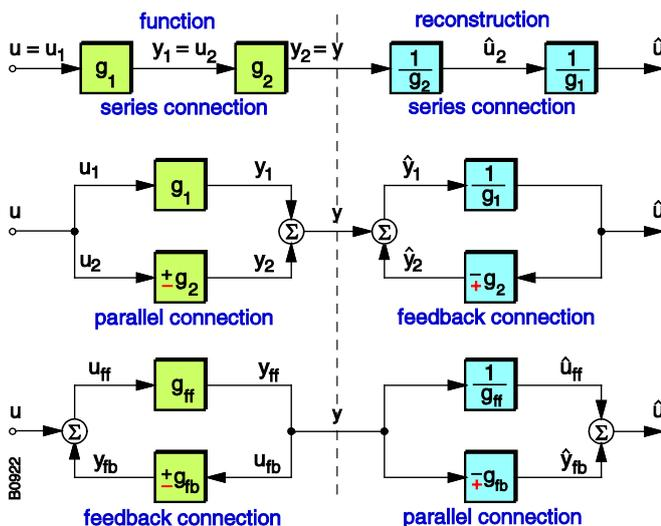
Figure 20. Reconstructed structures of the three connection types, series, parallel and feedback connection
