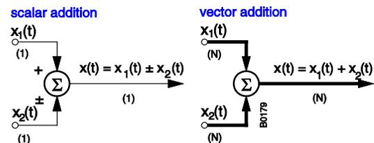
Figure 6. Linear signal connection
