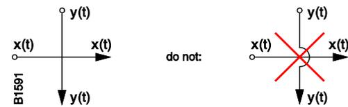
Figure 10. Crossing of signals and signal vectors in a signal relation diagram
