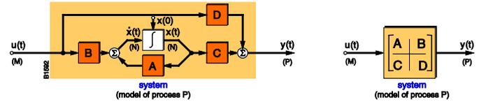
Figure 17: Canonical signal relation diagram of the linear, time invariant (LTI) dynamic system
