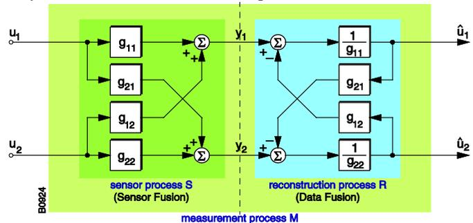
Figure 21. Inversion of the model of a sensor process with two input signals.
