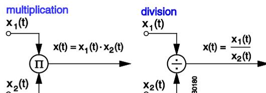
Figure 7. Nonlinear signal connection
