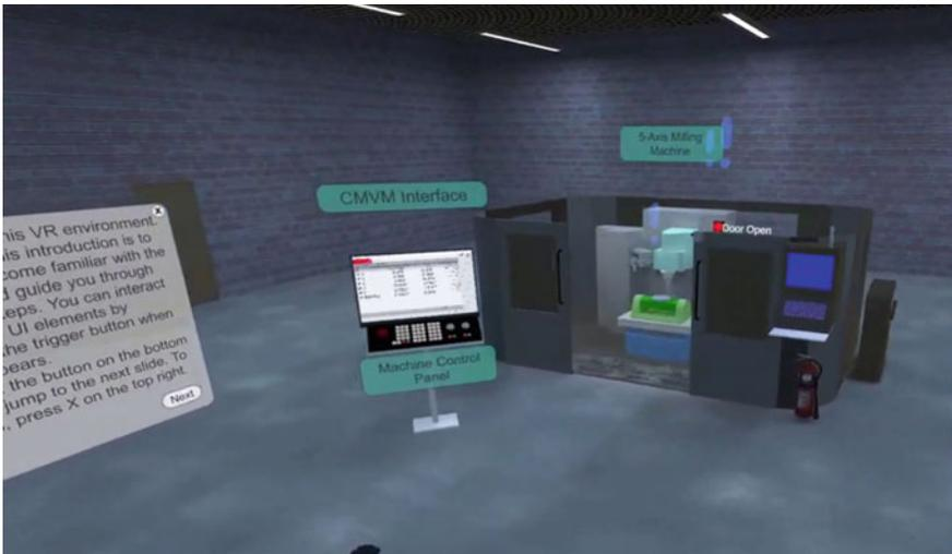
Fig. 3 The machine operator’s view in VR, including an assignment board on the left and the virtual machine tool including the virtualized machine control on the right
