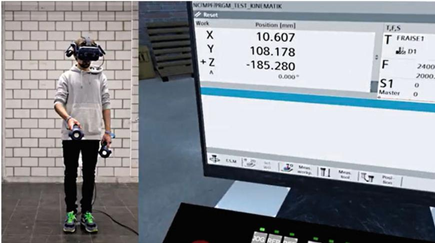
**Fig. 4** A machine operator accessing the machine's DT through VR (left) and a VR view of the virtualized Human-Machine Interface (HMI) (right)
